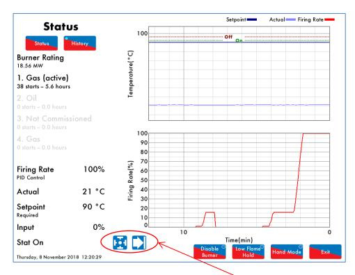
This data is logged for 24 hours on the MM. Use the scroll buttons to change the timescale of the data displayed, and press and drag on the axis to zoom in/out on the graph.
