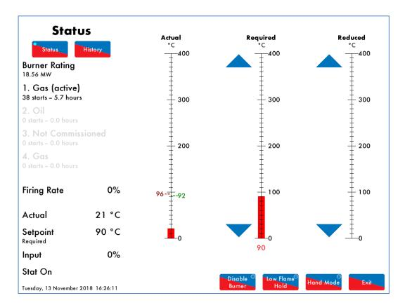
Press the up and down arrows to change the required or reduced setpoints (temperature for hot water boilers and pressure for steam boilers). If these arrows are not displayed, then either the user setpoint change has been disabled and/or an external setpoint is enabled by a climate computer (Fiduface).
