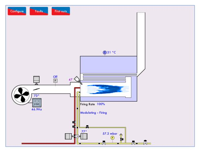
The Home screen displays the current boiler setup. It provides operation information for each component of the burner/boiler in real time. Pressing on a component triggers the display of further information.
